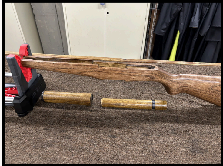
The wooden components of the M-1, after the coats have been stripped off.
